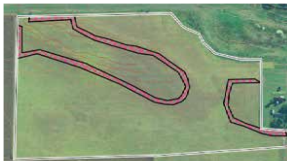
Field with two prairie strips on contour and additional strips on headlands.
