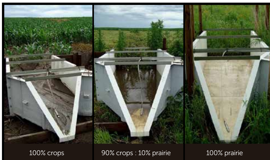
Figure 2: H-flumes comparing runoff between two STRIPS catchments (photo 1 and 2), and a nearby catchment in 100% prairie cover (photo 3). Photo: Iowa State University STRIPS
